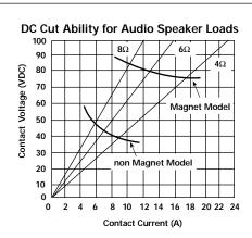
Note: This data is based on the max. allowable temperature for E type insulation coil (115°C).
